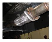
2. To remove your stock exhaust, unbolt the 2-bolt flange located in front of the muffler. For an easier removal of the factory exhaust cut off your tailpipe behind the muffler outlet. Leave all rubber grommets in place. Use WD-40 to aid in the removal of the hangers from the rubber grommets.
